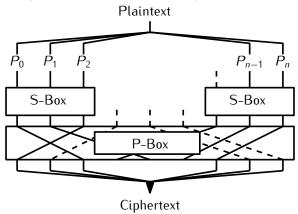
Built as a network of substitution/permutation functions:
